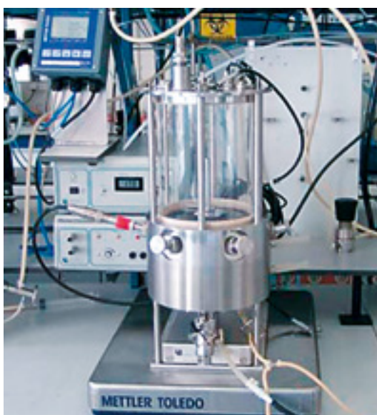
Fig. 1: 4.0 Liter laboratory fermenter with side-mounted CO 2 sensor.
