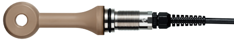
Figure 7: Inductive conductivity sensor with measuring coils and temperature sensor sealed within a polymer body
