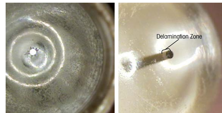
Figure 25 Cracked and delaminated anode/cathode
