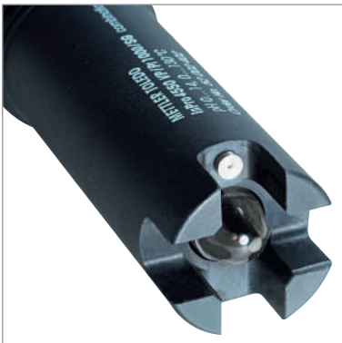
Slotted tip protects the pH glass membrane
