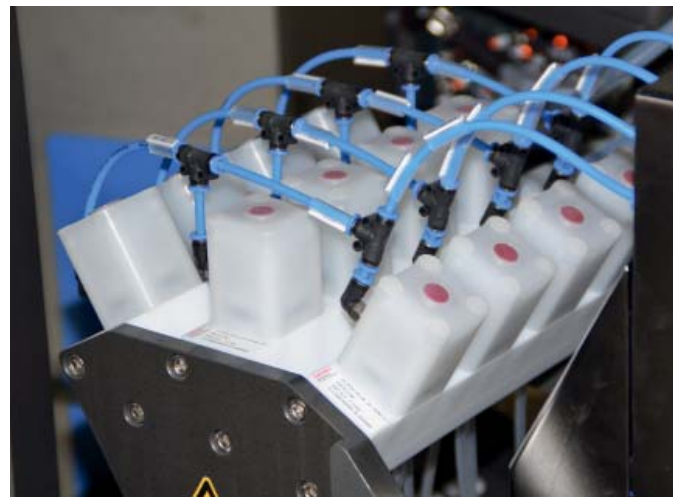
Multi-port valve block by GEMÜ with valves of the iComLine® series in the Harro Höfliger packaging machine
