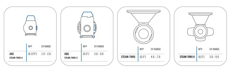
Cv values represent the approximate expected flow rate in gallons per minute of water at room temperature for a 1 PSI pressure drop. The flow is generally constrained by the smallest diameter, which in some cases will be the termination diameter and not the NFP.
