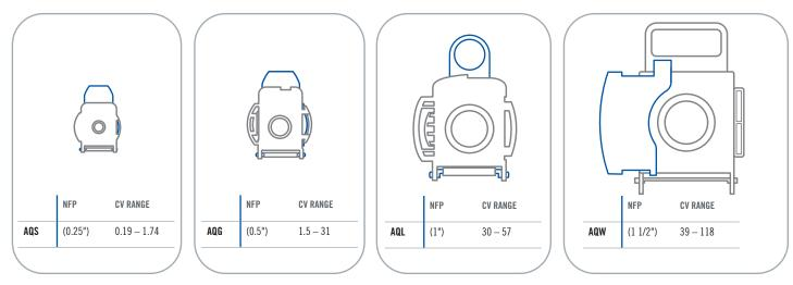
Cv values represent the approximate expected flow rate in gallons per minute of water at room temperature for a 1 PSI pressure drop. The flow is generally constrained by the smallest diameter, which in some cases will be the termination diameter and not the NFP.
