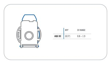
Cv values represent the approximate expected flow rate in gallons per minute of water at room temperature for a 1 PSI pressure drop. The flow is generally constrained by the smallest diameter, which in some cases will be the termination diameter and not the NFP.
