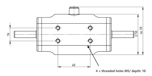
General construction with dimensions (sensor type with D8 connector, 8 mm outer and 4 mm inner diameter)
