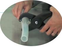
Specific cutting techniques are strongly recommended for APHP. The tubing must be cut with a chevron style cutter at a 90 degree angle to the tubing. View cutter product details at https://www.lislecorp.com/ specialty-tools/hose/hose-cutter.
