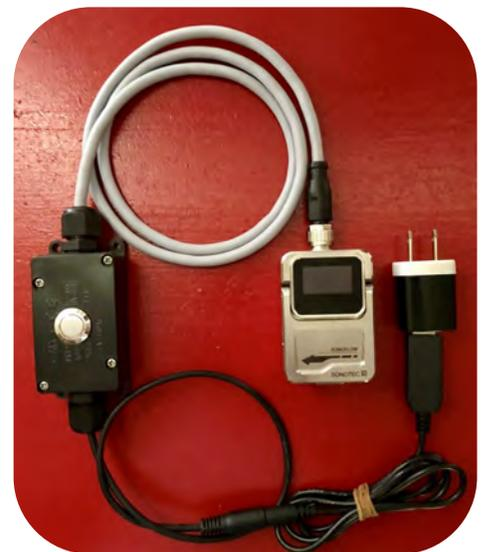
AC Power Cable with Auto Zero Switch (Sensor not included)
