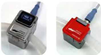
**Clamp on Sensors**—Flow rates from **20ml to 200 liters** per minute can be measured with good accuracy depending on sensor size, tubing type, and calibration. Always recommend the smallest tubing size possible relative to the flow rate. Custom low flow calibration required for average flows under 100 ml/min.
